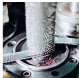
Patented high-speed machines cut, form and wrap aluminum fin stock around aluminum tubing.
