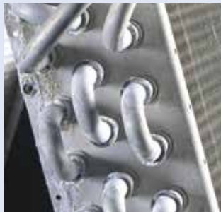
Aluminum tube and tube sheet after 500 hour salt spray.
