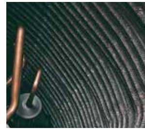
Spine Fin™ coils are fabricated in continuous lengths. Because of the number of leading edges, one row has the ability to transfer the same amount of heat as three rows of plate fin.
